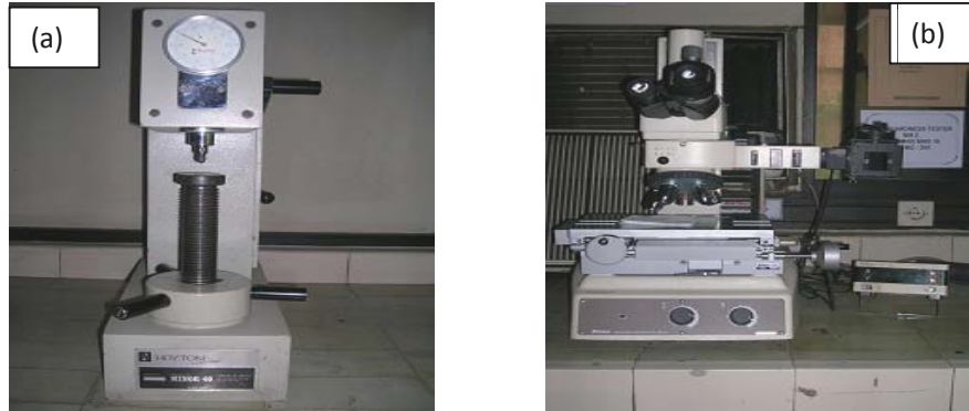
Gambar 3.7. Alat pengujian kekerasan: (a) mesin uji kekerasan metode Brinell Hoytom; (b) measuring microscope
