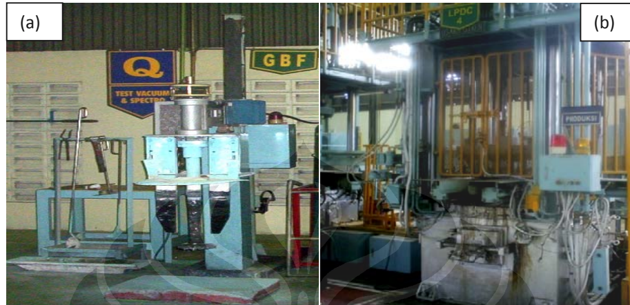
Gambar 3.2. a) GBF(Gas Bubbling Floatation); b) Mesin LPDC(Low Pressure Die Casting) dan Holding Furnace
